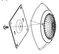
2. Make holes according to the manual. Put the plug into the hole first, and then install the screws.
