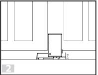
2. Fix the lock body onto the first moving side of the gate leaf, make sure there is at least 5 to 8 mm space between the stopper location hole surface & the bottom of lock body.
