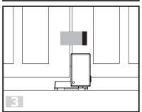
3. Install the stopper plate in corresponding position onto the same leaf which installed with lock DS218, this is to make sure when 2 leaves are closed, the stopper plate can limit the leaf which cannot opened either.
